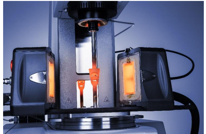
Figure 10: The CTD 1000 with three-point-bending (TPB) geometry
