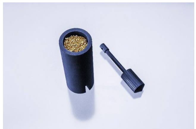
Figure 2: Carbon measuring geometry with a profiled cylinder
