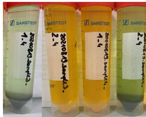
Fig. 3: Samples KZ03 (2 vessels from left) and KZ04 (2 vessels from right) with acid mix μ~4 digested at different temperatures. Both greenish solutions with heavy grey residue to the left and right reached only 230°C, while the clear, orange solutions in the middle reached a digestion temperature of 250°C.
