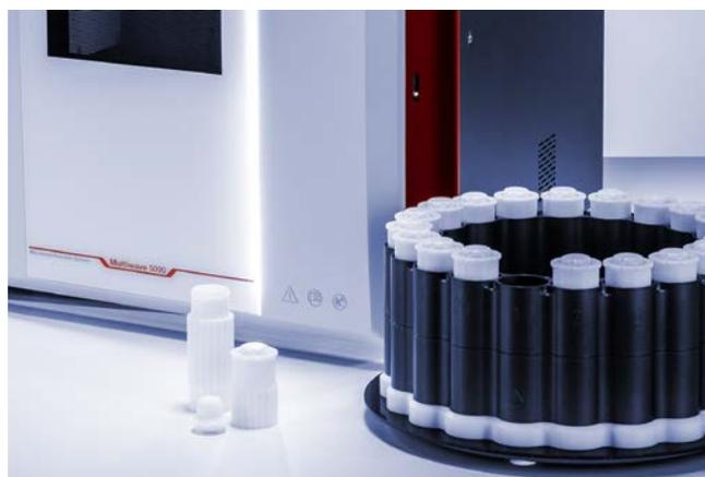
Fig. 1: Rotor 20SVT50 and Multiwave 5000
